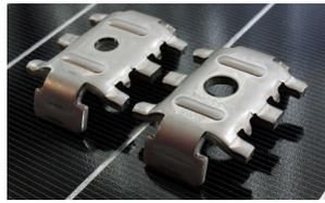
The BMCSS integrated bonding mid-clamps are made of corrosion resistant 304 stainless steel, which makes them a durable, long lasting and reliable solution for all environments. The down-turned points are designed to pierce the anodized coating of the module frame. The result is excellent conductivity bonding the PV modules together. Essentially, the modules become one singular piece of metal, creating a clear electrical path to the ground.
